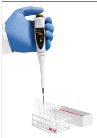
Hold the pipette in a vertical position during aspiration.
